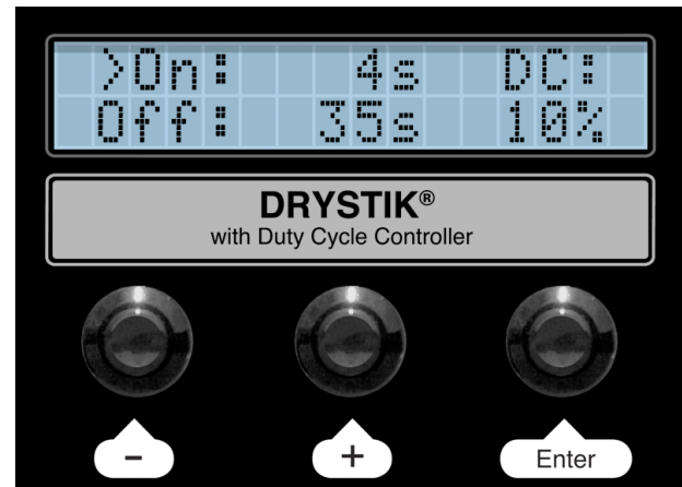
Fig. 9 DRYSTIK ADS-2 button functions labeled on device faceplate
