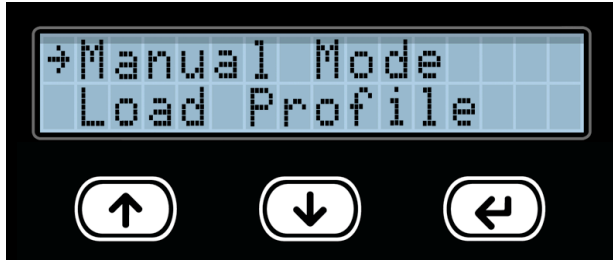
Fig. f The ADS-3 menu is navigated using the [↑], [↓], and [Enter] buttons
