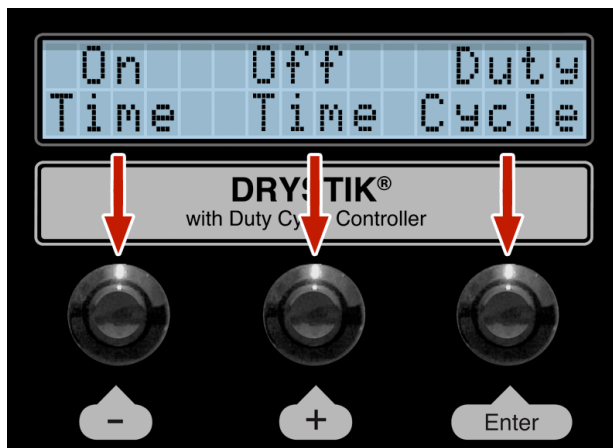
Fig. 8 DRYSTIK ADS-2 button functions labeled on LCD display
